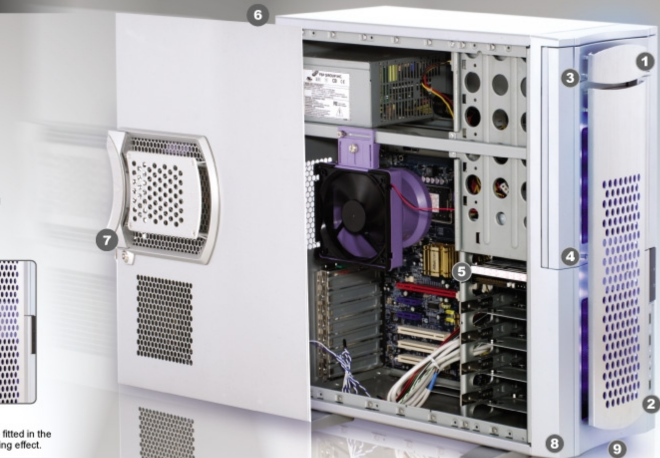
7 Lockable sidepanel. Lockable easy to open and close sidepanel.
